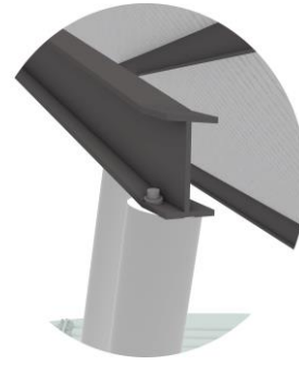
COLUMN TO BEAM (ROOF)
